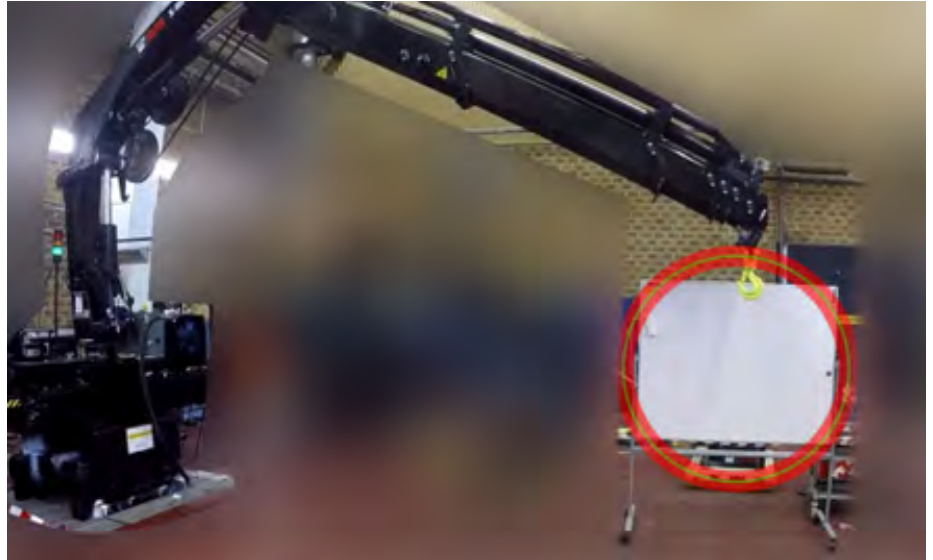
Figure 5: A HIAB loader crane following a circle trajectory using feedforward controllers trained from data [4]. See full video in this link
