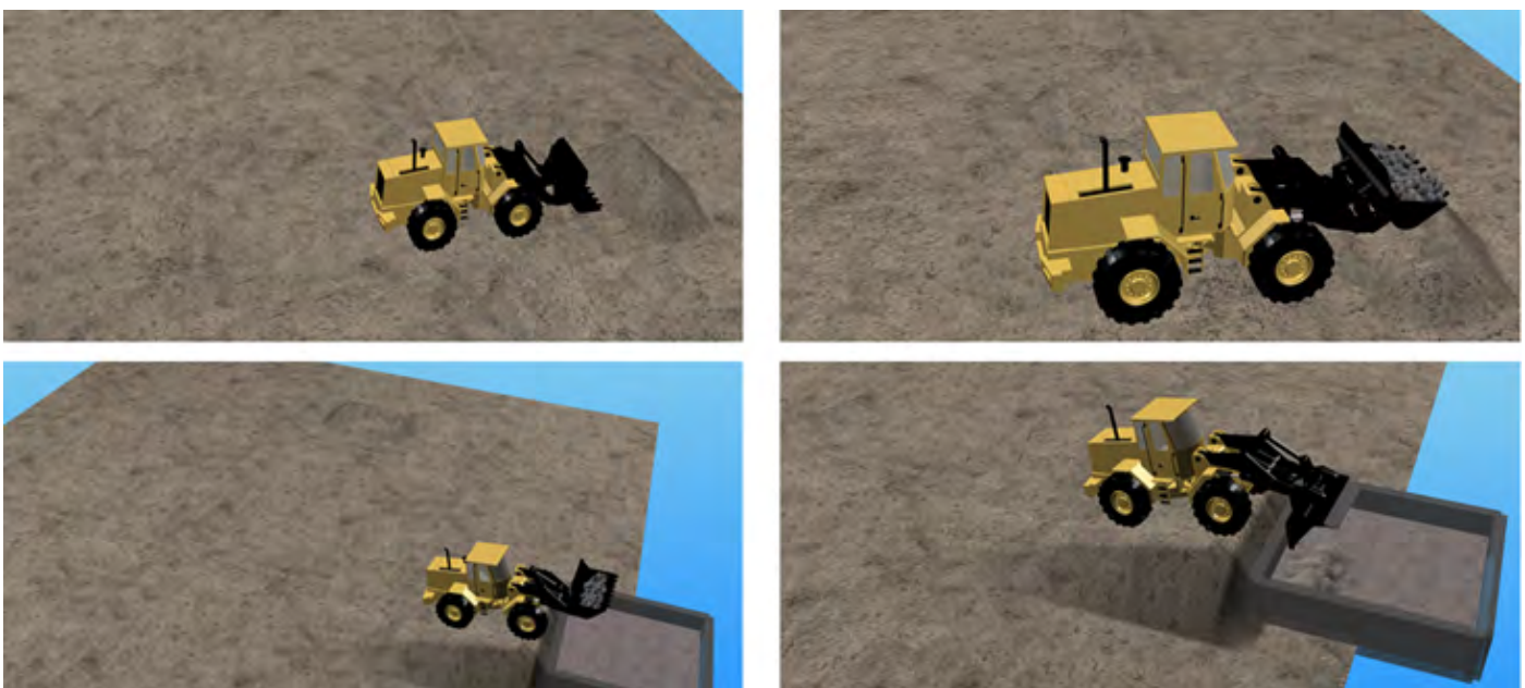
Figure 3: Loading and dumping sequences performed by an autonomous machine.
