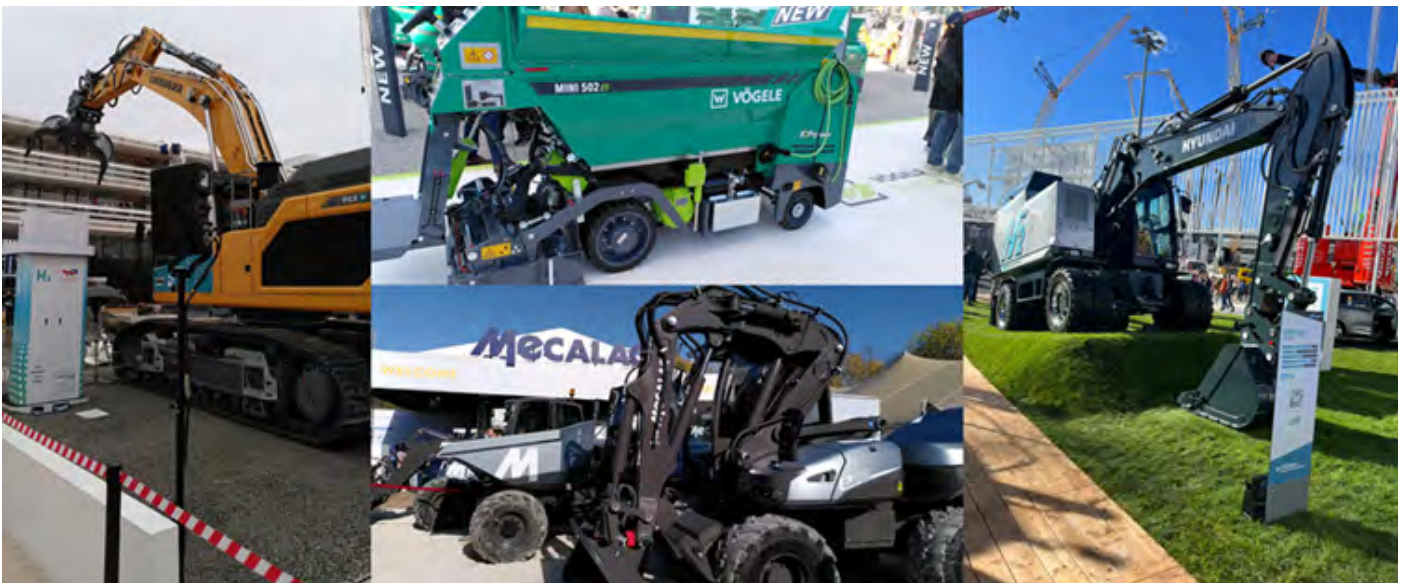
Figure 1: Photos taken by David Fassbender at Bauma 2022: Left, excavator with hydrogen combustion engine; top center, road paver with electro-mechanical actuators; lower center, battery electric machines in the 10 tonne class; and right, excavator with hydrogen fuel cell.
